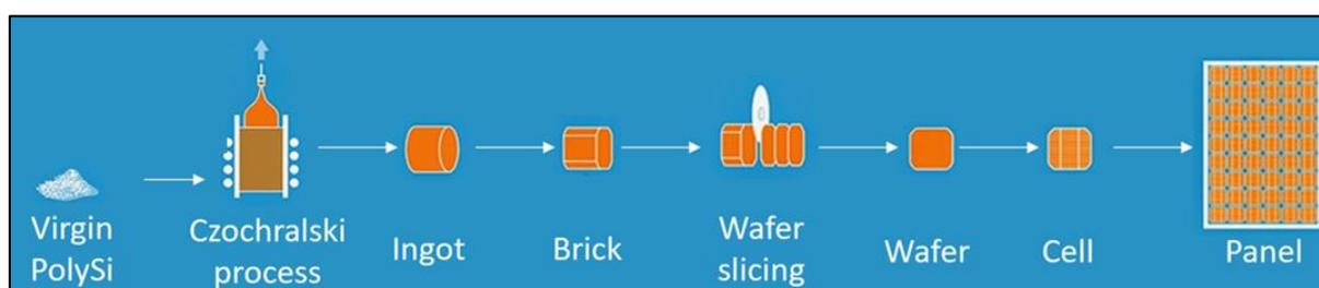
Step 1 - **PolySi**: The raw material used to produce the cells is a high purity silicon called “Solar grade silicon” or “PolySi”.
