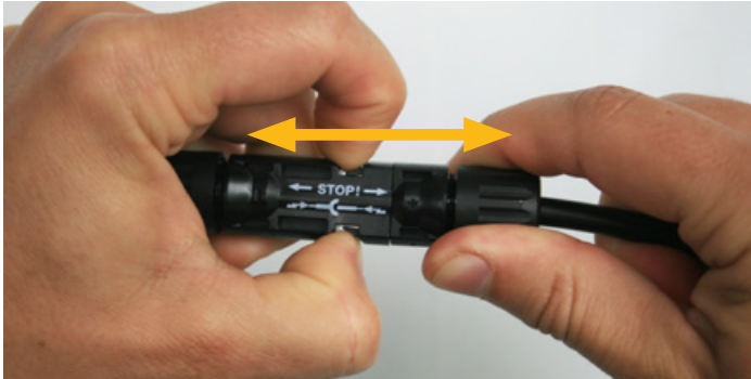
Fig. 4: Disconnecting an MC4 type connector with tool (Multi-Contact or Hosiden)
