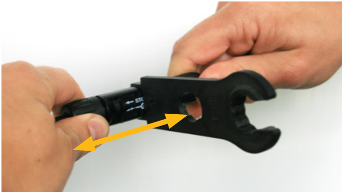
Fig. 4: Disconnecting an MC4 type connector with tool (Multi-Contact or Hosiden)
