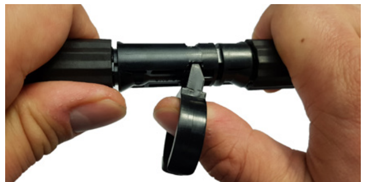
Fig. 8: Disconnecting MC4 Evo2 and Tonglin connectors
