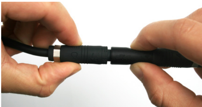
Fig. 5: Connection of Radox connectors showing ~2 mm gap
