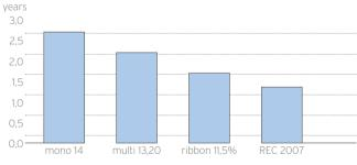
Figure 2. Energy Pay-Back time (in years) of solar systems for the three main silicon-based PV technologies in 2005 compared to REC 2007. The solar systems are assumed installed in Southern Europe, with about 1700 sun hours per year.
