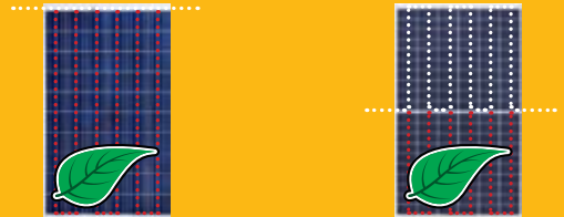
When one half of a standard module is shaded, none of the module produces electricity
