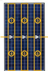
**Standard Module** With three internal strings of cells
