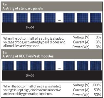
This advantage is best seen in installations where inter-row shading can cause the system to stop generation (fig. 4). By splitting the REC TwinPeak into two sections, the string will continue to produce electricity in at least 50% of the panel until the other section is also shaded (fig. 3b) improving the overall energy yield.
