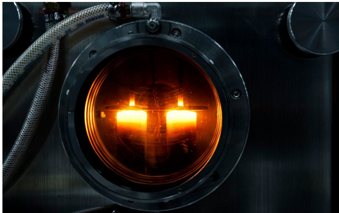
Img. 1: Industrial production of solar silicon in a Siemens reactor, showing the intense levels of heating required.
