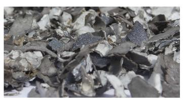
Img. 6: Recovered plastics from a solar module, including backsheet, ready for recycling (Butenhoff Werbeagentur & Verlag).
